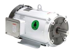
Leeson Washguard White Duck premium efficiency AC induction motor, washdown and inverter rated, 10hp, 3-phase, 230/460 VAC, 1800rpm, TEFC, NEMA 215TC frame, rolled steel, C-face/rigid base mount.
