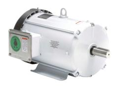
Leeson Washguard White Duck premium efficiency AC induction motor, washdown and inverter rated, 10hp, 3-phase, 230/460 VAC, 1800rpm, TEFC, NEMA 215T frame, rolled steel, rigid base mount.
