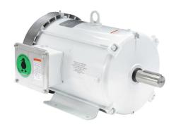
Leeson Washguard White Duck premium efficiency AC induction motor, washdown and inverter rated, 7-1/2hp, 3-phase, 230/460 VAC, 1800rpm, TEFC, NEMA 213T frame, rolled steel, rigid base mount.
