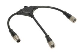
IDEM T-port, (1) 8-pin male M12 quick disconnect to (2) 8-pin female M12 disconnects. For use with IDEM Z-Range switches.
