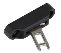
IDEM actuator tongue (key), flexible mounting tab with 40mm mounting hole spacing mount, 316 stainless steel. For use with IDEM MK1 and INCH series safety switches.
