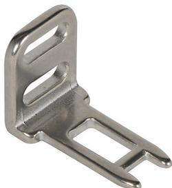
IDEM actuator tongue (key), 90 degree mounting tab with 8mm mounting hole spacing mount, 316 stainless steel. For use with IDEM MK1 and INCH series safety switches.
