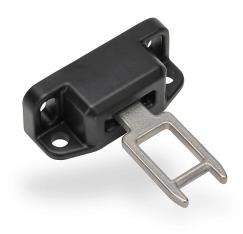
IDEM actuator tongue (key), black aluminum heavy duty flexible mounting tab with 40mm mounting hole spacing mount, 316 stainless steel. For use with all IDEM K-SS, KM, KM-SS, KP and K-15 series safety switches.
