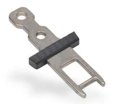
IDEM actuator tongue (key), straight mounting tab with 20mm mounting hole spacing mount, 316 stainless steel. For use with all IDEM K-SS, KM, KM-SS, KP and K-15 series safety switches.
