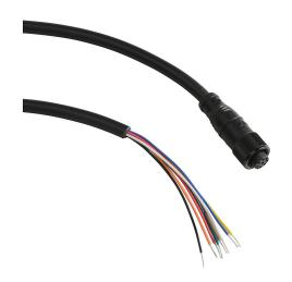
IDEM connection cable, 8-pin female axial M12 quick-disconnect to pigtail, 16.4ft/5m cable length.
