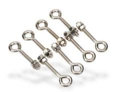
IDEM eye bolt, galvanized steel, 84mm length, M8 x 1.25 threads. Package of 8. For use with cable-pull safety switches.
