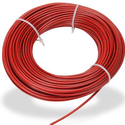
IDEM pull cable, 164ft/50m cable length, 4mm diameter, galvanized steel, plastic jacket, red. For use with cable-pull safety switches.
