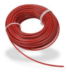
IDEM pull cable, 98.4ft/30m cable length, 4mm diameter, galvanized steel, plastic jacket, red. For use with cable-pull safety switches.
