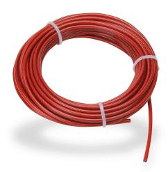
IDEM pull cable, 32.8ft/10m cable length, 4mm diameter, galvanized steel, plastic jacket, red. For use with cable-pull safety switches.
