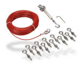
IDEM pull cable kit, 98.4ft/30m cable length, 4mm diameter, stainless steel. For use with cable-pull safety switches.
