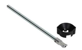
Socomec shaft, 320mm length,  $10 \times 10$ mm. For use with S1 and S2 type handles. Shaft alignment guide 14290000 included.
