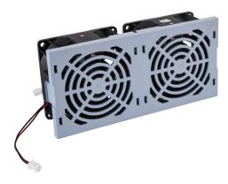
WEG Electric CFW500 series main cooling fan, replacement,  $80 \times 38$  mm, 24 VDC. For use with WEG CFW500 series E frame AC drives.
