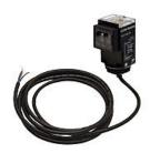
Eaton photoelectric sensor, rectangular, diffuse, infrared, 10ft sensing distance, selectable light-on/dark-on, SPDT EM relay, potentiometer, 66 Hz switching frequency, plastic housing, pigtail.
