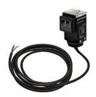
Eaton photoelectric sensor, rectangular, diffuse, infrared, 10ft sensing distance, selectable light-on/dark-on, solid state relay, potentiometer, 500 Hz switching frequency, plastic housing, pigtail.
