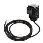
Eaton photoelectric sensor, rectangular, diffuse, infrared light emission, 10ft sensing distance, selectable light-on/dark-on, solid state relay, potentiometer, 500 Hz switching frequency, plastic housing, pigtail.
