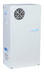
Pfannenberg DTS 3141 air conditioner, 4100 BTU/H, R-134a, 115 VAC operating voltage, carbon steel housing, RAL 7035 light gray, filter-free, side mount. For use with NEMA/UL Type 12 enclosures.
