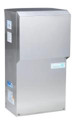
Pfannenberg DTS 3181 air conditioner, 4100 BTU/H, R-134a, 115 VAC operating voltage, 304 stainless steel housing, filter-free, side mount. For use with NEMA/UL Type 4 & 4X enclosures.
