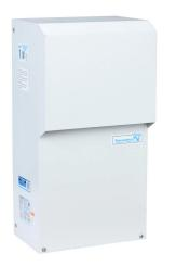
Pfannenberg DTS 3161 air conditioner, 4100 BTU/H, R-134a, 460 VAC operating voltage, carbon steel housing, RAL 7035 light gray, filter-free, side mount. For use with NEMA/UL Type 3R & 4 enclosures.
