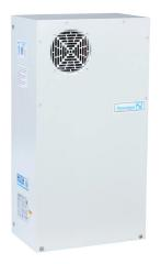
Pfannenberg DTS 3141 air conditioner, 4100 BTU/H, R-134a, 460 VAC operating voltage, carbon steel housing, RAL 7035 light gray, filter-free, side mount. For use with NEMA/UL Type 12 enclosures.
