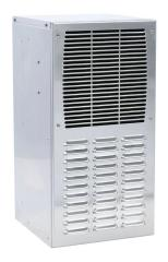
Pfannenberg DTS 3081 air conditioner, 2700 BTU/H, R-134a, 115 VAC operating voltage, 304 stainless steel housing, filter-free, side mount. For use with NEMA/UL Type 4 & 4X enclosures.
