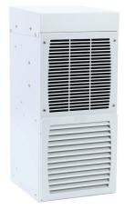
Pfannenberg DTS 3041 air conditioner, 2700 BTU/H, R-134a, 460 VAC operating voltage, carbon steel housing, RAL 7035 light gray, filter-free, side mount. For use with NEMA/UL Type 12 enclosures.
