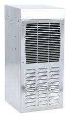
Pfannenberg DTS 3081 air conditioner, 2700 BTU/H, R-134a, 460 VAC operating voltage, 304 stainless steel housing, filter-free, side mount. For use with NEMA/UL Type 4 & 4X enclosures.
