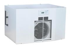
Pfannenberg DTT 6801 air conditioner, 14000 BTU/H, R-134a, 460 VAC operating voltage, carbon steel housing, RAL 7035 light gray, filter-free, top mount. For use with NEMA/UL Type 12 enclosures.
