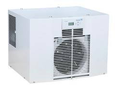
Pfannenberg DTT 6401 air conditioner, 7100 BTU/H, R-134a, 460 VAC operating voltage, carbon steel housing, RAL 7035 light gray, filter-free, top mount. For use with NEMA/UL Type 12 enclosures.
