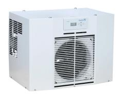
Pfannenberg DTT 6201 air conditioner, 3570 BTU/H, R-134a, 460 VAC operating voltage, carbon steel housing, RAL 7035 light gray, filter-free, top mount. For use with NEMA/UL Type 12 enclosures.
