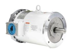
Leeson Washguard White Duck premium efficiency AC induction motor, washdown and inverter rated, 5hp, 3-phase, 230/460 VAC, 1800rpm, TEFC, NEMA 184TC frame, rolled steel, C-face mount.
