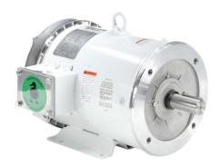
Leeson Washguard White Duck premium efficiency AC induction motor, washdown and inverter rated, 5hp, 3-phase, 230/460 VAC, 3600rpm, TEFC, NEMA 184TC frame, rolled steel, C-face/rigid base mount.
