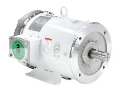
Leeson Washguard White Duck premium efficiency AC induction motor, washdown and inverter rated, 5hp, 3-phase, 230/460 VAC, 3600rpm, TEFC, 184TC frame, rolled steel, C-face/rigid base mount.
