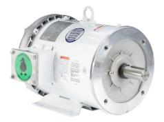
Leeson Washguard White Duck premium efficiency AC induction motor, washdown and inverter rated, 3hp, 3-phase, 230/460 VAC, 1800rpm, TEFC, NEMA 182TC frame, rolled steel, C-face/rigid base mount.
