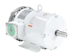
Leeson Washguard White Duck premium efficiency AC induction motor, washdown and inverter rated, 5hp, 3-phase, 230/460 VAC, 1800rpm, TEFC, NEMA 184T frame, rolled steel, rigid base mount.
