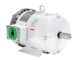
Leeson Washguard White Duck premium efficiency AC induction motor, washdown and inverter rated, 3hp, 3-phase, 230/460 VAC, 1800rpm, TEFC, 182T frame, rolled steel, rigid base mount.
