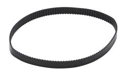
SureMotion timing belt, 0.08in MXL pitch, 1/4in wide, 130 tooth, 10.4in pitch length (circumference), polyurethane, polyester reinforced. Package of 3.
