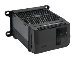
Stego enclosure heater, axial fan, 200W heating capacity, high performance cartridge heating element, 24 VDC operating voltage, adjustable thermostat with external sensor connection, N.C. (open on rise) -4 to 104 deg F, 35mm DIN rail or panel mount.
