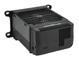
Stego enclosure heater, axial fan, 200W heating capacity, high performance cartridge heating element, 24 VDC operating voltage, adjustable thermostat, N.C. (open on rise) -4 to 104 deg F, 35mm DIN rail or panel mount.
