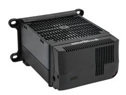
Stego enclosure heater, axial fan, 200W heating capacity, high performance cartridge heating element, 24 VDC operating voltage, adjustable thermostat, N.C. (open on rise) -4 to 104 deg F, 35mm DIN rail or panel mount.
