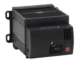
Stego enclosure heater, axial fan, 1200W heating capacity, PTC resistor heating element, 230 VAC operating voltage, 50/60 Hz, adjustable thermostat, N.C. (open on rise) 0 to 60 deg C, 35mm DIN rail or panel mount.
