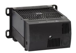
Stego enclosure heater, axial fan, 950W heating capacity, high performance cartridge heating element, 120 VAC operating voltage, 50/60 Hz, 35mm DIN rail or panel mount.
