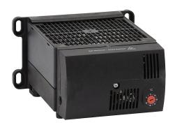
Stego enclosure heater, axial fan, 950W heating capacity, high performance cartridge heating element, 230 VAC operating voltage, 50/60 Hz, adjustable thermostat, N.C. (open on rise) 0 to 60 deg C, 35mm DIN rail or panel mount.
