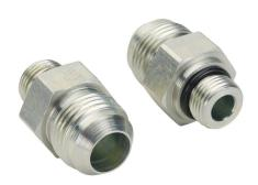
HY-TECH hydraulic fluid adapter, straight, plated steel body, (1) -12 male JIC 37 deg and (1) -8 male o-ring boss. Package of 2.
