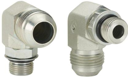
HY-TECH hydraulic fluid adapter, elbow, plated steel body, (1) -12 male JIC 37 deg and (1) -8 male o-ring boss. Package of 2.
