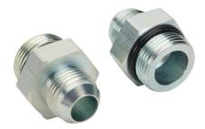
HY-TECH hydraulic fluid adapter, straight, plated steel body, (1) -12 male JIC 37 deg and (1) -16 male o-ring boss. Package of 2.
