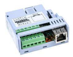
WEG Electric CFW500 series communication module, Profinet, Modbus TCP, Modbus RTU and BACnet, 2 ports, (1) Profinet (RJ45) and (1) RS-485 (3-pin terminal) port(s). For use with WEG CFW500 series AC drives.
