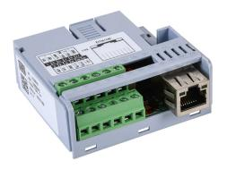
WEG Electric CFW500 series communication module, Modbus TCP, Modbus RTU and BACnet, 2 ports, (1) Ethernet (RJ45) and (1) RS-485 (3-pin terminal) port(s). For use with WEG CFW500 series AC drives.
