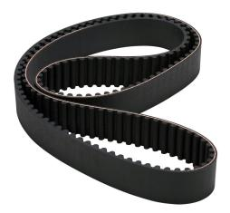
SureMotion timing belt, 8mm 8M pitch, 30mm wide, 160 tooth, 1280mm pitch length (circumference), neoprene, fiberglass reinforced.
