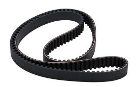
SureMotion timing belt, 8mm 8M pitch, 20mm wide, 160 tooth, 1280mm pitch length (circumference), neoprene, fiberglass reinforced.
