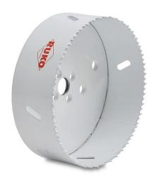
RUKO bi-metal hole saw, 4-3/4in (121mm), 8% cobalt high-speed steel (HSSE-Co8), hardened steel backer, fine tooth, 1.5in (38mm) maximum cutting depth.
