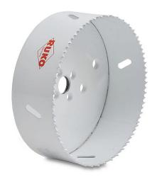
RUKO bi-metal hole saw, 4-3/4in (121mm), 8% cobalt high-speed steel (HSSE-Co8), hardened steel backer, fine tooth, 1.5in (38mm) maximum cutting depth.
