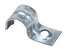
Minerallac 1-hole conduit mount strap, standard duty, UL Type UL 1565. Package of 100. For use with 1/2in OD tubing or cable, 12-3, 10-2, 10-3 BX armored cable, 8 AWG SER, 3/8in FMC.
