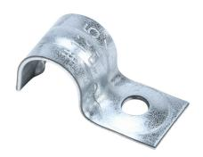
Minerallac 1-hole conduit mount strap, standard duty, UL Type UL 1565. Package of 25. For use with 1/2in OD tubing or cable, 12-3, 10-2, 10-3 BX armored cable, 8 AWG SER, 3/8in FMC.
