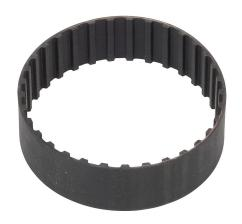
SureMotion timing belt, 3/8in L pitch, 1in wide, 33 tooth, 12.4in pitch length (circumference), neoprene, fiberglass reinforced.
